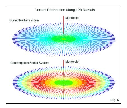
The currents in the buried radials begin at a relatively low level and continually decrease along the length of the radials. Because buried radials are in a medium of limited conductivity and significant relative permittivity, the current distribution is not the same as in wires in air. The level of segmentation
