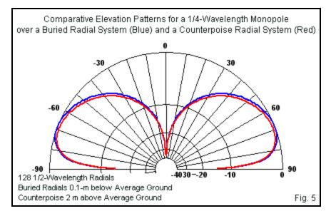
**Fig. 5** overlays elevation patterns for the two monopole installations. Both patterns have a TO elevation angle of 21 degrees. The buried-radial system yields a maximum gai of 2.24 dBi, while the counterpoise system shows a maximum gain of 1.93 dBi, about a 0.3-dB difference. One might change the counterpoise system gain by solidifying the radial structure, perhaps with cross wires linking the radials, especially in the outer regions in which the radials show maximum separation.
