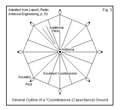
See **Fig. 3** for a sketch adapted from Laport's volume. My version is simplified in omitting the antenna control box ("tuning house" below the wires) and, more significantly, in only showing a few of the wires that make up the counterpoise system. As Laport notes, the counterpoise system is preferable to a buried radial system in terms of loss reduction in the AM broadcast band. However, for ground-
